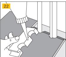
**HEATING PIPES:** Watch the picture carefully how to cut a Parky board. It is important to follow the instructions to achieve a nice result. Around the pipes you can finish the floor with silicone. It is important that the expansion gap is closed off to avoid moisture in the Parky floor. **(Pic. 21 & 22)**
