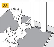
**HEATING PIPES:** Watch the picture carefully how to cut a Parky board. It is important to follow the instructions to achieve a nice result. Around the pipes you can finish the floor with silicone. It is important that the expansion gap is closed off to avoid moisture in the Parky floor.
