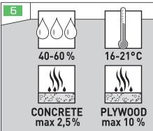
**STORAGE**: Store Par-ky floors in a perfectly dry and protected room with an air humidity of 40 to 60% and a temperature of 16 to 21° C (61-70° F). In order to prevent deformation, the boxes may not come into contact directly with the ground. Warning: Do not open the boxes until the moment of installation.
