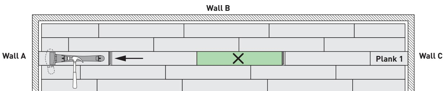
8. Now, to unlock the long side of the planks: Return to the row beside the damaged plank, and starting near Wall C, attach the tool to Plank 2 as close to the wall as possible and tap the tool towards Wall B (closest wall) until the two planks partially disengage. Repeat along this row every 30 cm/12 inch until the long side of the damaged plank is totally exposed.
