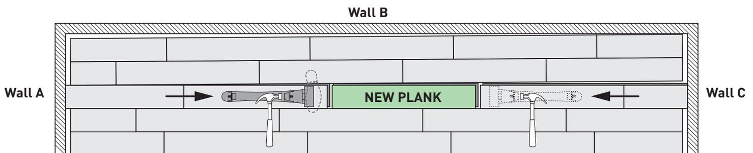
10. Next, re-engage all the long sides, starting by the planks nearest to Wall A. The repair is complete when all joints are re-engaged.
