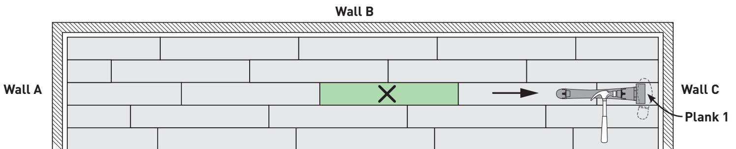
6. Continue in the same method, unlocking planks on that row, until you reach the damaged plank.
