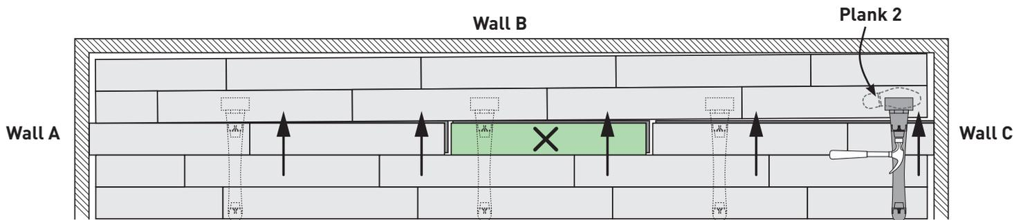
9. Remove the damaged plank and click the new plank into place. Lock together the short sides of the replaced plank, continuing along the full row until all short sides are re-engaged.
